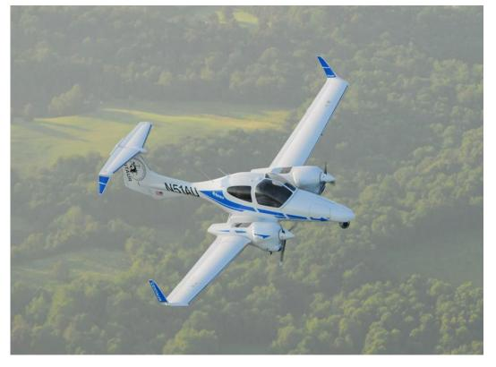
Centaur provides a versatile airborne sensing platform for a range of mission types including defense, intelligence, law enforcement, and environmental research. Centaur can be operated from a remote ground control station, with or without an onboard pilot.
